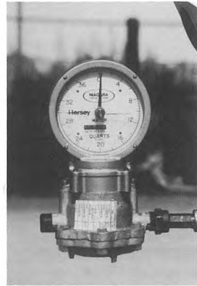
Batch Style — Water Meter Manual or Automatic
